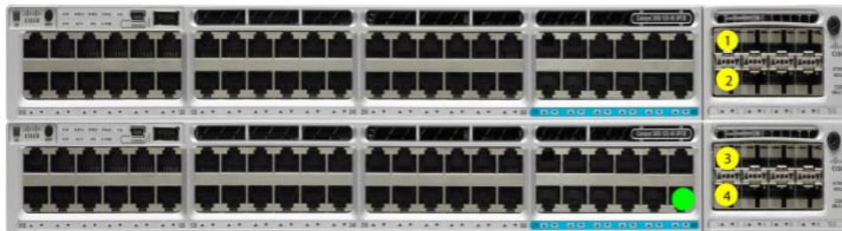
Dual 10GE + ToR Switches (standalone or stacked)
