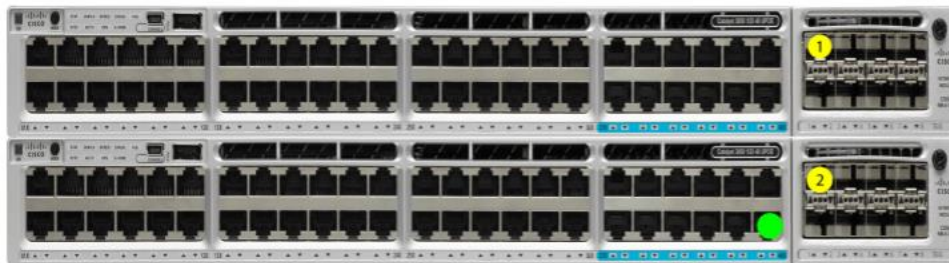
Dual 10GE + ToR Switches (standalone or stacked)
