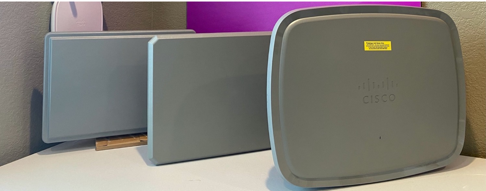
Three generations of High-Density WiFi Stadium Antennas
