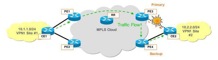
CEF (via BFD or link layer mechanism) detects PE3-CE2 link failure
