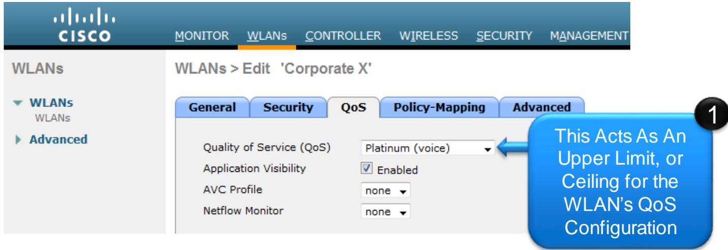
The screenshot shows the Cisco WLAN configuration interface for 'Corporate X'. The 'QoS' tab is selected, and the 'Quality of Service (QoS)' dropdown is set to 'Platinum (voice)'. A blue callout box with a '1' in a black circle points to the dropdown menu, containing the text: 'This Acts As An Upper Limit, or Ceiling for the WLAN's QoS Configuration'.
