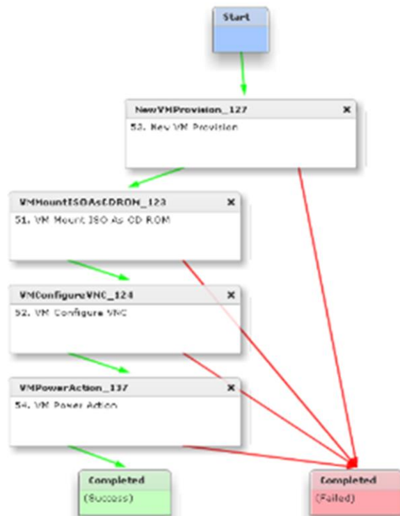
Workflow to provision VMWare Virtual Machine using ISO Image
