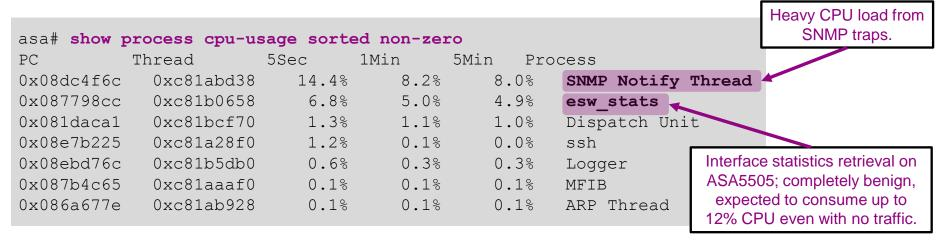
Use cpu profile under TAC supervision for per-function load granularity
