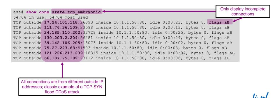
ASA protects the server from SYN flood by responding with a TCP SYN ACK to validate the client before permitting the connection to the protected server
