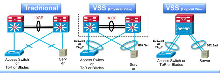
Simplifies operational Manageability via Single point of Management, Non-loop design, minimise reliance on STP, eliminate FHRP etc
