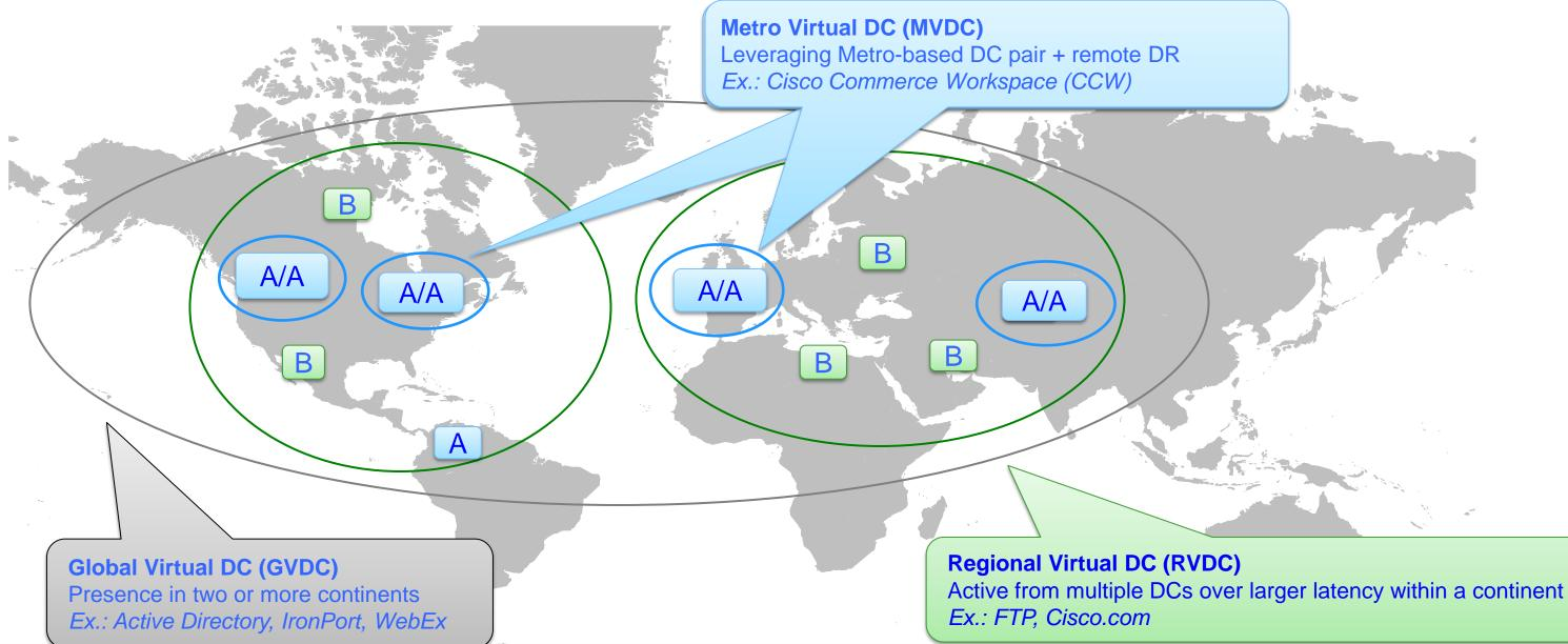
Distributed Virtual Data Centre (DVDC) Architecture Three Variations Reflecting Varying Latency Constraints and Performance Requirements
