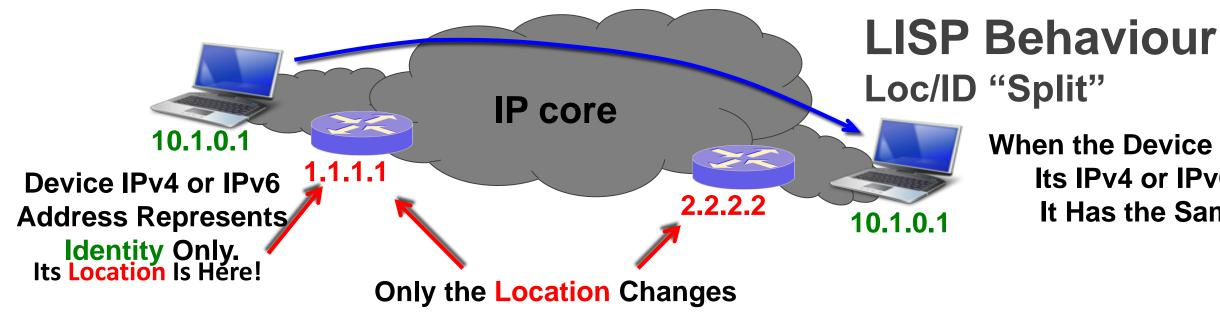
When the Device Moves, It Gets a New IPv4 or IPv6 Address for Its New Identity and Location
