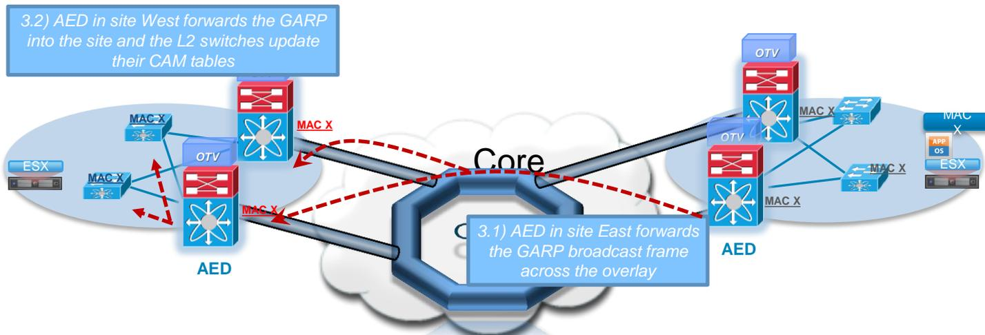
Note: GARP is used as example traffic, same behaviour is achieved with any other L2 broadcast frames exchanged
