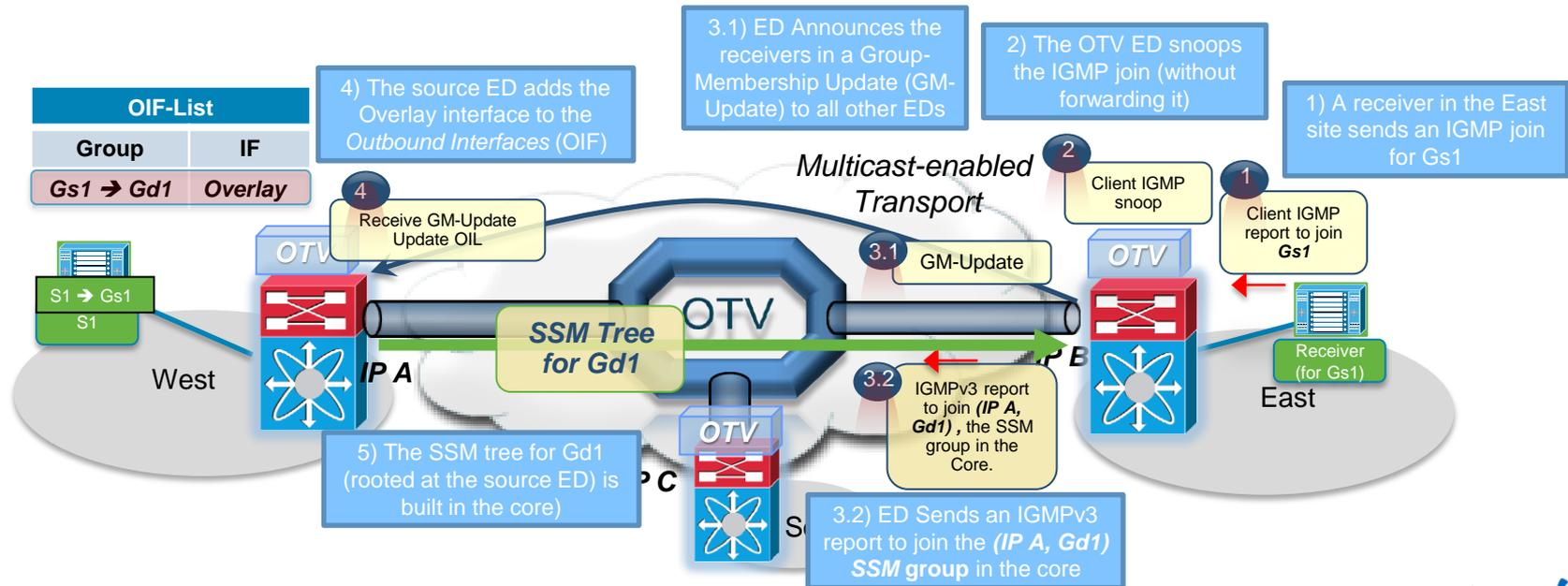
It is important to clarify that the edge devices join the core multicast groups as hosts, not as routers!
