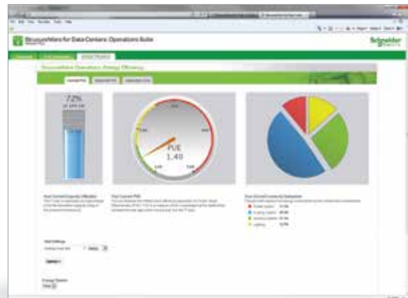
Full insight into current and historical energy efficiency for facilities identifies efficiency losses and enables improved PUE/DCiE values at subsystem level
