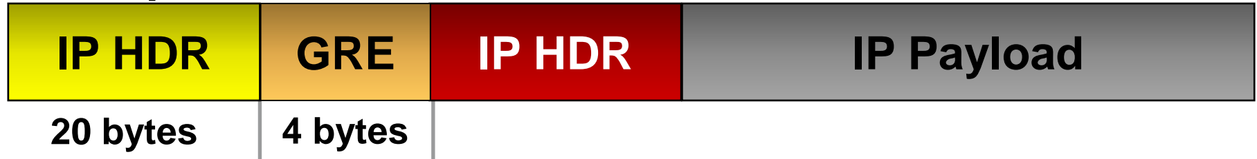
GRE packet with new IP header: Protocol 47 (forwarded using new IP dst)
