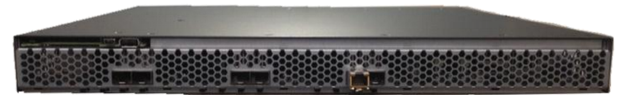
Next-Generation WLAN Controller (5760)
